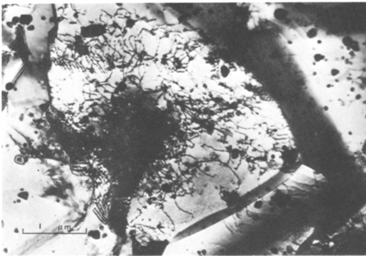
Figure 4 The microstructure of a specimen deformed to 10% at 823 K in Region III.
