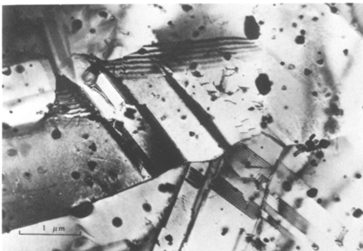
Figure 5 The microstructure of a specimen deformed to 10% at 823 K in Region II.
